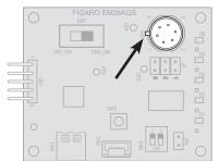
Ensure that the sensor is inserted so that the protrusion on the sensor base is facing the 5-Pin connector.
