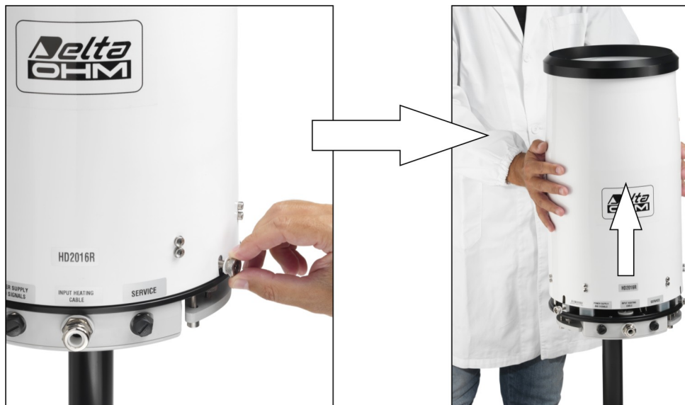
Fig. 9.2: removing the cylindrical cover
