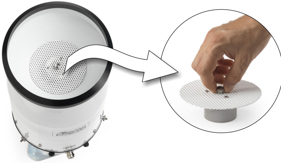
Fig. 9.1: removing the upper filter
