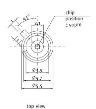
UVA-only SiC based UV photodiode A = 0,50 mm<sup>2</sup>
