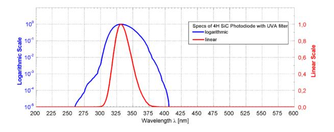
UVA-only SiC based UV photodiode A = 0,20 mm<sup>2</sup>
