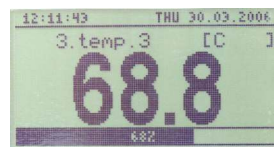
the current value of the measurement signal The height of the digits: 18 mm
